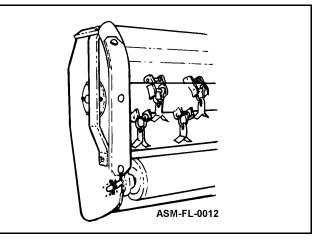
**ACAUTION** If it is necessary to loosen the nut on the pivot pin. Re-torque the nut to 400 ft labs. Failure to do so will cause the nut to loosen during use, allowing the pin to come out, thereby causing certain machine damage.
